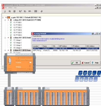
The e.bloxx series is designed for industrial and experimental test systems requiring precise high speed measurement of electrical, thermal and mechanical quantities in engine- and component test beds.
